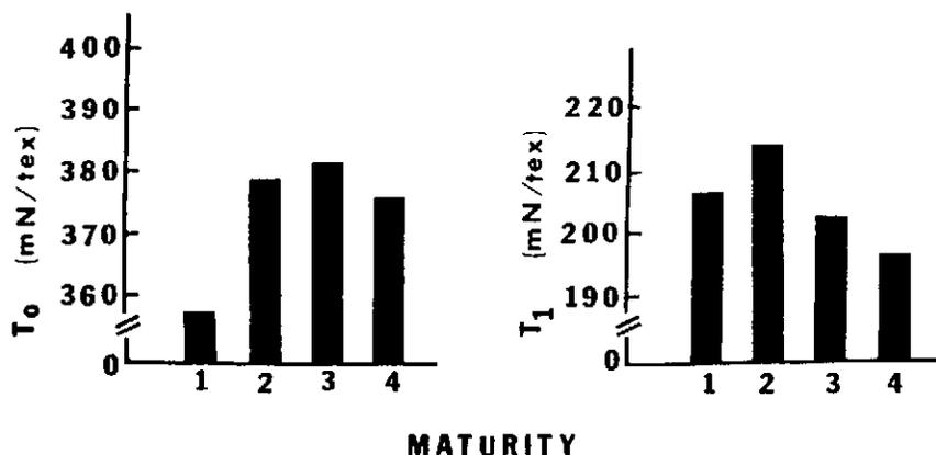
Figure 1. The tenacity of cotton fibers of four maturities.  $T_0$  is the tenacity in flat bundle tests where the clamping jaws are closely appressed, zero gauge.  $T_1$  is the tenacity in flat bundle tests where the clamping jaws are spaced 3.2 mm apart. The maturities 1, 2, 3 and 4 are 1.27, 1.94, 2.48 and 2.59  $\mu\text{m}$  wall thicknesses, respectively. (Data from Ramey *et al.*, 1982.).
